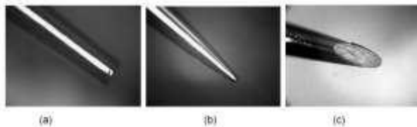
Figure-2: (a) Flat (b) Conical with Rounded (c) Wedged Electrode
