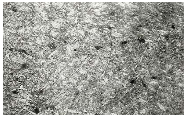
Figure-2: Typical Microstructure of the weld metal (Heat input 843.37 J / mm)
